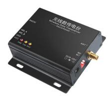
E3A-DTU-1W is a 433M wireless transceiver (with RS232/485 interfaces) with transparent transmission, operates at 425-450.5MHz (default: 433MHz), the operating voltage is 8V ~ 28V.
