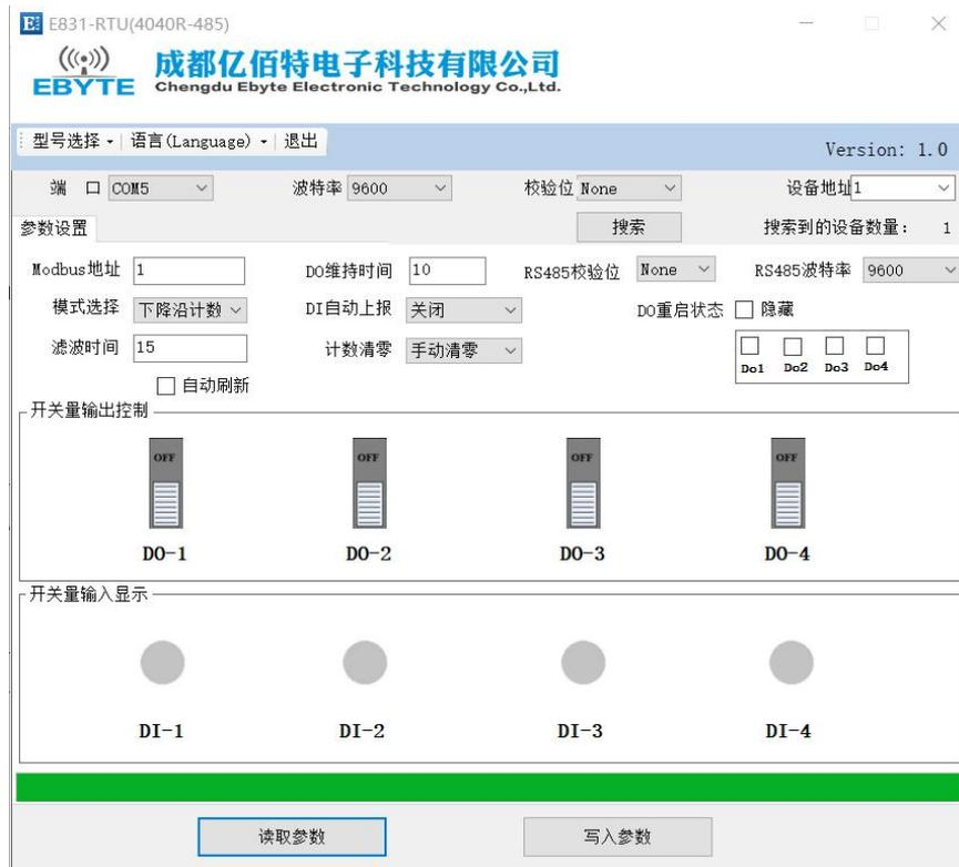
Tick Auto Refresh to read and configure the input and output ports.
