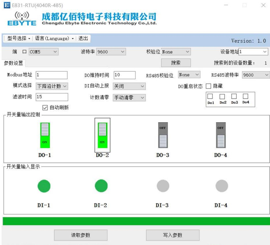
Note: Do not tick Auto refresh when reading or writing parameters. Instead, tick it after configuration or reading is completed, otherwise the parameter writing or reading may not be successful.
