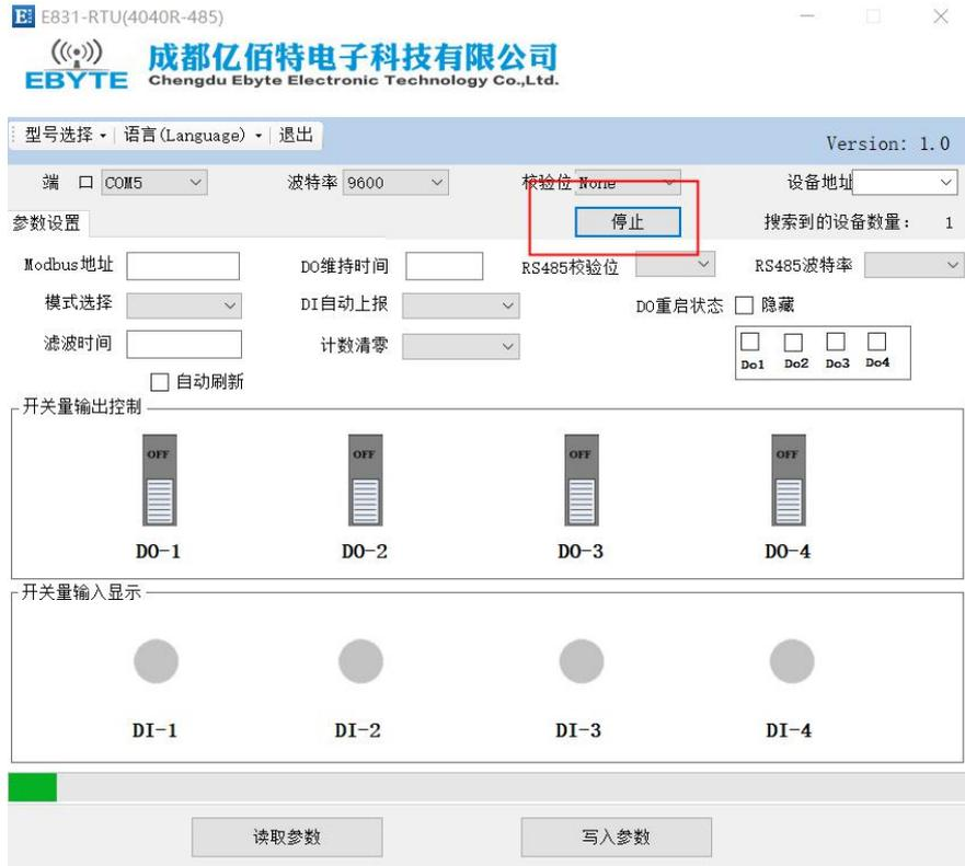
At this point, users can see the device address of the current device. Click on read parameters or write parameters to read parameters and configure parameters.
