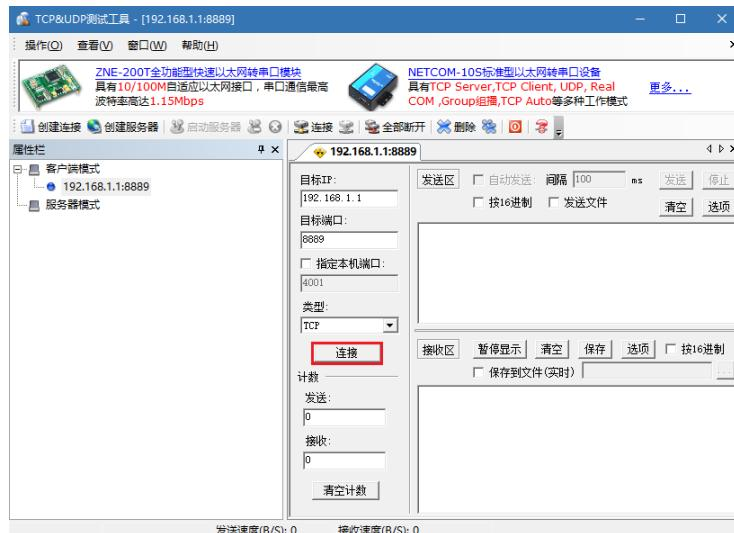
③. The **LINK indicator** on the baseboard will be lit up, it means connection is completed, then the PC and the module can communicate with each other mutually (it means TCP & UDP testing tool and AccessPort can communicate with each other mutually), if not, please redo above steps.
