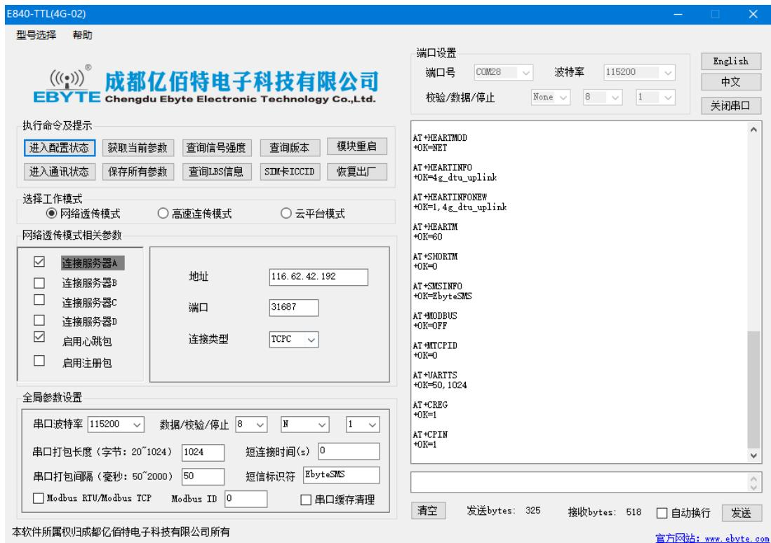
2. Query the signal strength, set the device connection server IP and port number to be: 116.62.42.192, 8124; (Ebyte test server), and finally click "Save all parameters", and finally as shown below::
