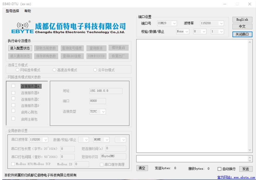
1. Click the tool "Enter Configuration Status" button and wait for the device parameters to be automatically obtained. After completion, the following figure is displayed::
