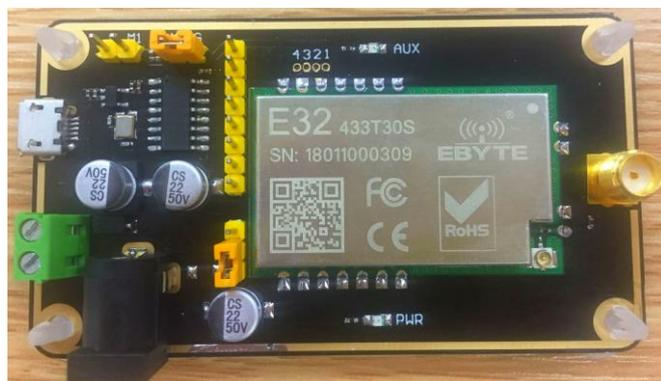
As shown above , connect to jumpers ( 5V power supply , mode 1 ) , see function details from E22 UART
