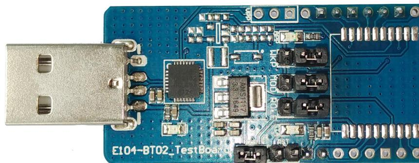
E104-BT02-TB test board adapts USB interface, which can quickly sets the Bluetooth related features and functions
