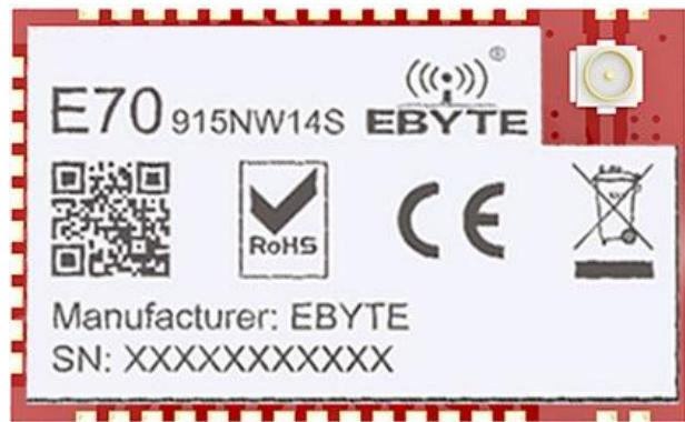
E70-915NW14S is the first 915MHz wireless module that solves a series of problems caused by traditional modules. Users will spend less effort to deal with complex network protocols, which greatly reduces the difficulty of customer development and shortens the user's development period. The protocol guarantees the stability and packet rate of the entire wireless communication system.
