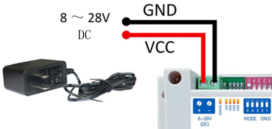
Figure 2-2-1 Power wiring diagram
