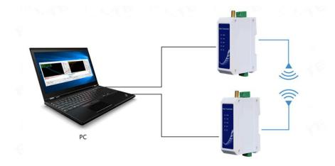
4 Start two serial port debugging assistants, select the serial port baud rate to be 9600bps (default), and the check method to be 8N1 to make serial port transparent transmission.
