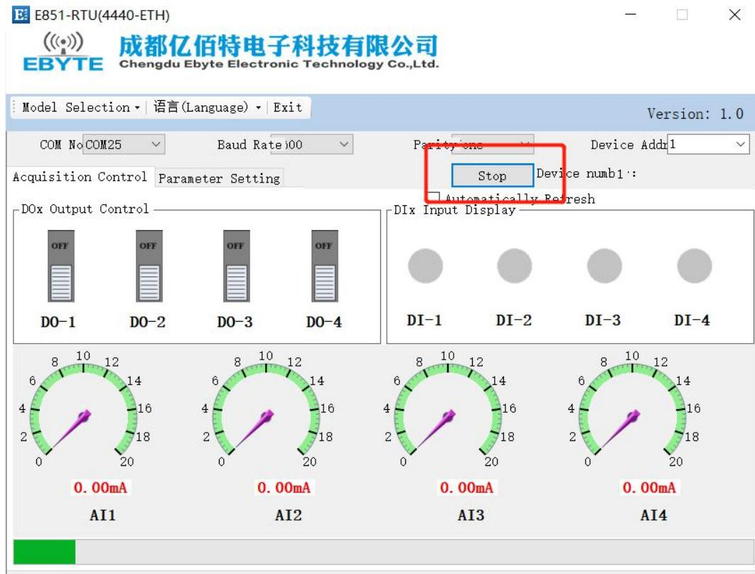
At this time, the device address of the current device can be seen, and the "auto refresh" processing can be performed, and the switch output control, the digital input read, and the differential analog input can be read.
