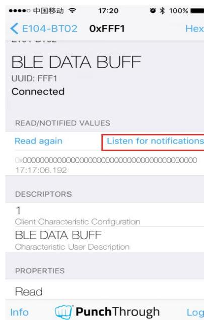
4. Use COM debugging assistant and transmit character string "1234567890" via module E104-BT02 (operating in wake-up transparent transmission mode). APP says character string is received.
