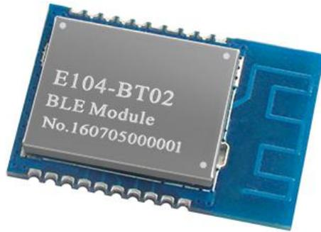
E104-BT02 is a SMD 1mW (0dBm) wireless UART to BLE module with high cost performance, small size and embedded PCB antenna and operates at 2.4 GHz frequency band. Serial port (UART) can be used to receive and transmit Bluetooth data, which lowers the threshold to apply Bluetooth.
