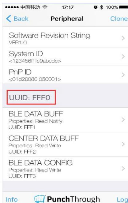
3. Display 3 channels and FFF1 is channel for data transmission from module to master. Enter this channel and click "Listen for notifications" .
