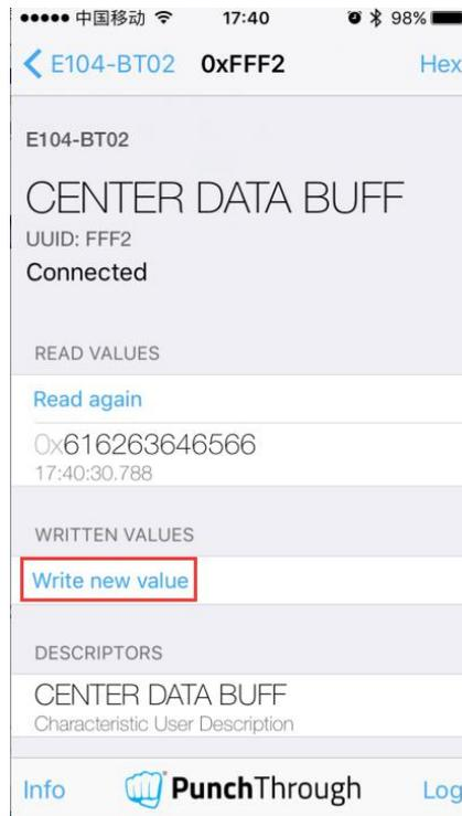
6. Fill out and transmit "abcdef" , module E104-BT02 will output received data via UART transparent transmission.
