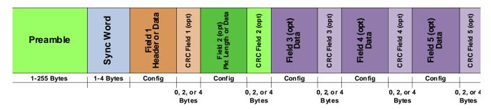
Figure 12. Packet Handler Structure
