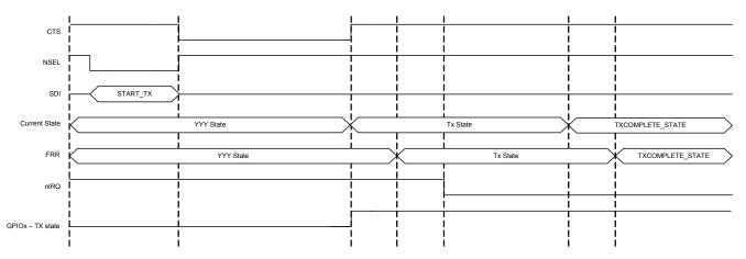
Figure 6. Start\_TX Commands and Timing
