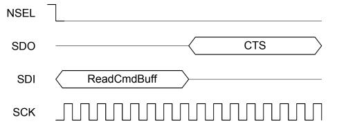
Figure 2. SPI Read Command—Check CTS Value
