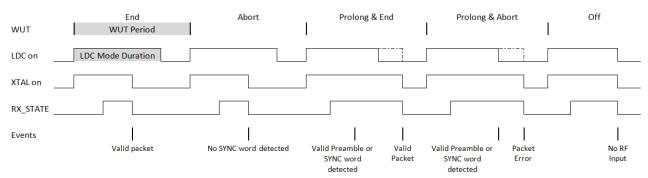
Figure 14. Low Duty Cycle Mode for RX
