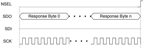
Figure 3. SPI Read Command—Clock Out Read Data
