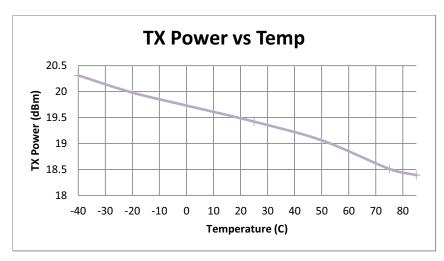
Figure 9. +20 dBm TX Power vs. Temp
