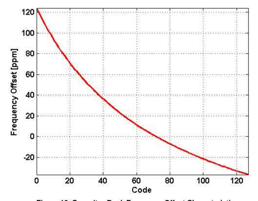
Figure 10. Capacitor Bank Frequency Offset Characteristics
