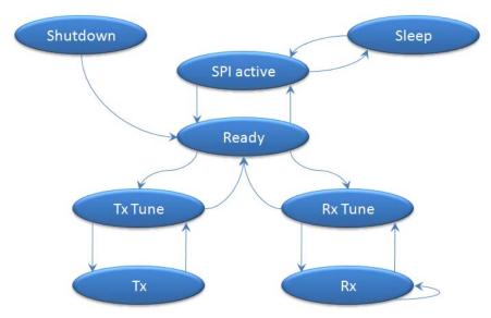
Figure 4. State Machine Diagram
