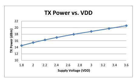
Figure 8. +20 dBm TX Power vs. VDD
