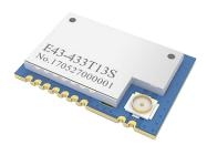
E43-433T13S is a wireless rf module with super high cost performance designed by Chengdu Ebyte. It has 4 operating mode and 2 transmitting methods, which has it's own characteristics, suitable for various application. With strict testing before factory, E43-433T13S perfectly supports the industrial application, ensuring the reliability and the consistency of batch production.
