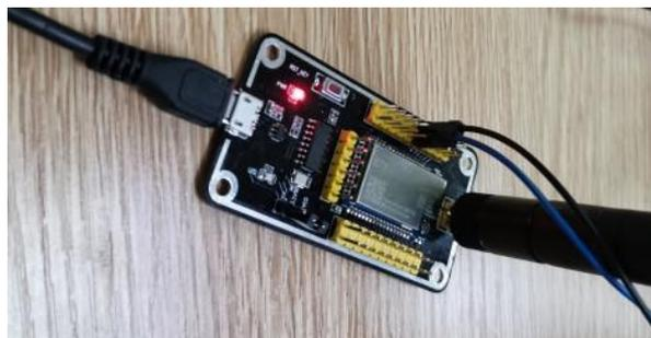
For secondary development, you are recommended to use test kit [E78-900TBL-01A](#). It is convenient and efficient. First, power the module through the serial port of the test kit, and then connect the NRST pin and SWIM pin of ST-LINK to the test kit to download the program. As shown above.
