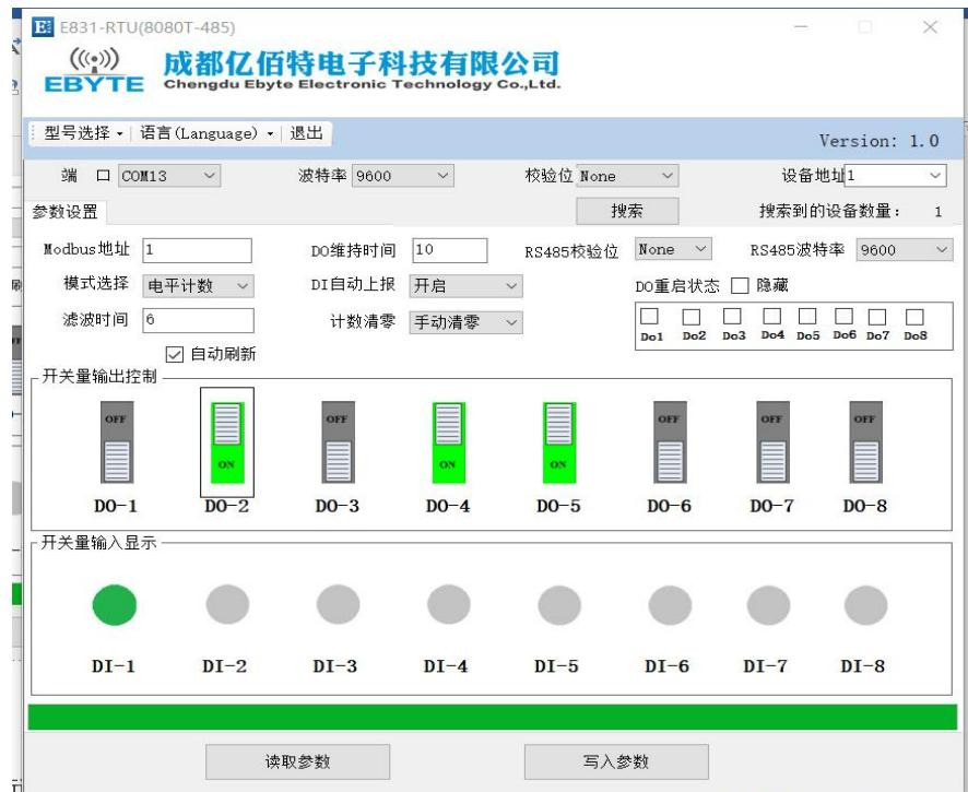
Note: Do not select automatic refresh when reading or writing parameters. Select automatic refresh after configuration or reading is completed, otherwise the parameter writing or reading may not be successful.
