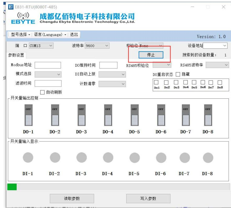
At this time, you can see the device address of the current device. Click on read parameters or write parameters to read parameters and configure parameters.
