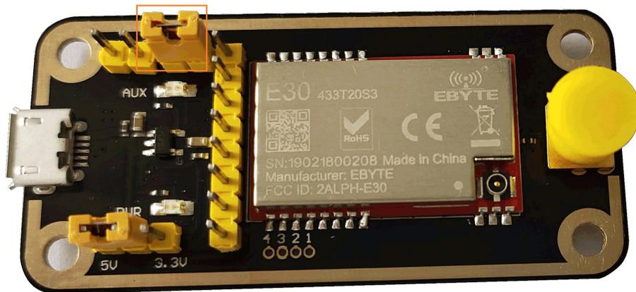
As shown above, connect to jumpers (5V power supply, mode 1 ) see function details from E30 UART module manual.
