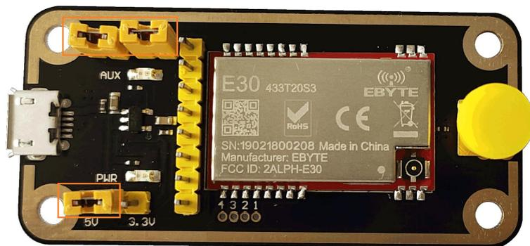
As shown above connect to jumpers(5V power supply, mode 0 ), both E30-433TBL-0 are configured this way, open serial port, for data TX and RX, and AUX indicator is blinking.
