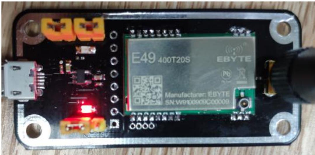
As shown in the picture, plug in the jumper cap and select 5V power supply or 3.3V to power the module. Both E49-400TBL-01 are configured in this way, open the corresponding serial port to receive and send data.
