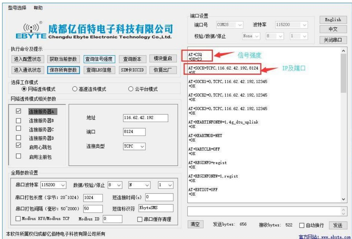
5. Click the tool "Module Restart" button and wait for the device LINK light to be on.
