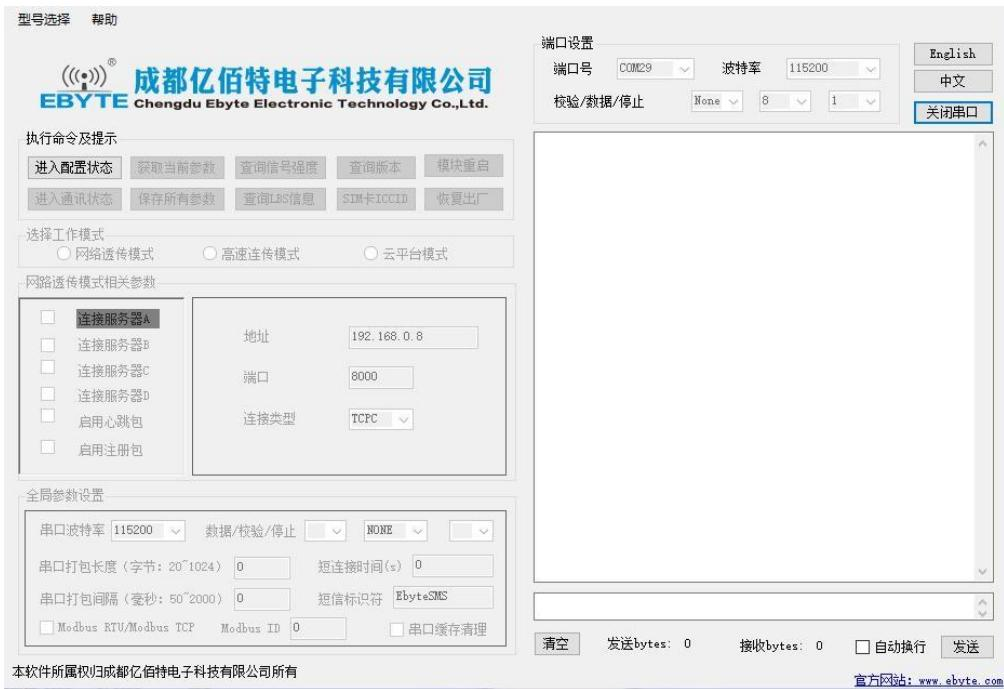
3. Click the tool "Enter Configuration Status" button and wait for the device parameters to be automatically obtained. After completion, the following figure is displayed::
