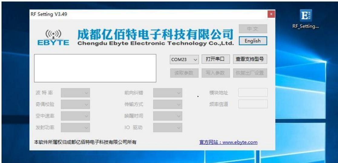
3. Open the serial port tool and use the file sending method to open RF\_Setting3.49.exe. After the device is connected to the network server normally, click “send file” and the sending is completed as shown below. :
