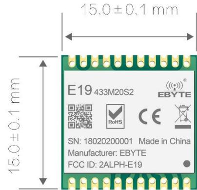
Since the module is a pure RF transceiver module, you need to use the MCU driver or a dedicated SPI debug tool.
