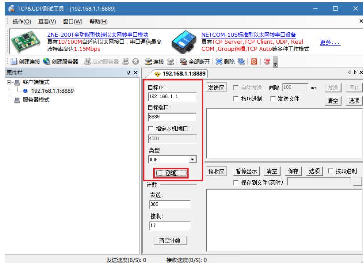
⑦. When creation is completed, it can realize two-way transmission between PC and server (it means transmission between TCP&UDP testing tool and AccessPort), if not, please redo above steps.
