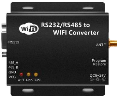
E103-W02-DTU is a UART-WiFi server supporting RS232/RS485 to WiFi two-way transparent transmission, it enables the UART device to immediately have TCP/IP network interface function, which extends the operation range of the device.
