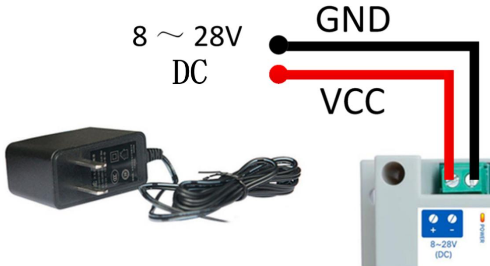
Fig 2-2-1 Power supply wiring diagram
