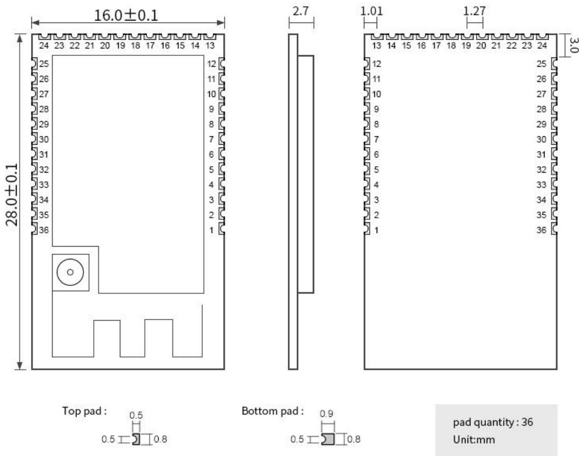
Figure 3-1 Mechanical size and pin definition
