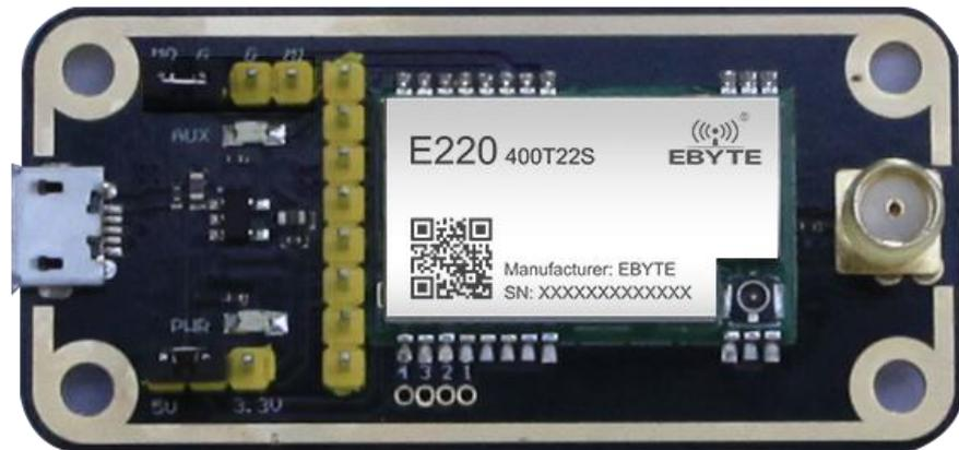
As shown above , connect to jumpers ( 5V power supply , mode 2 ) , see function details from E22 UART module manual.
