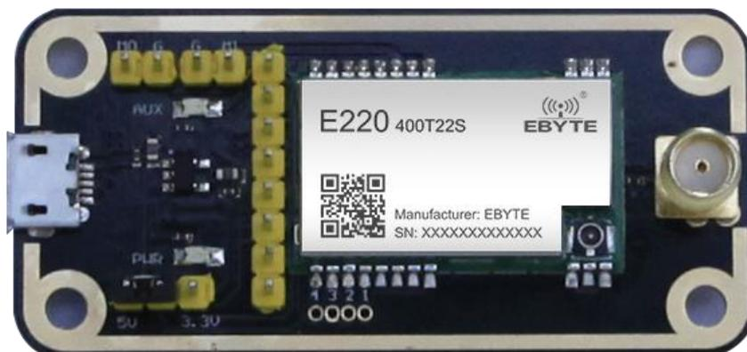
As shown above , connect to jumpers ( 5V power supply , mode 3 ) , see function details from E22 UART module manual.
