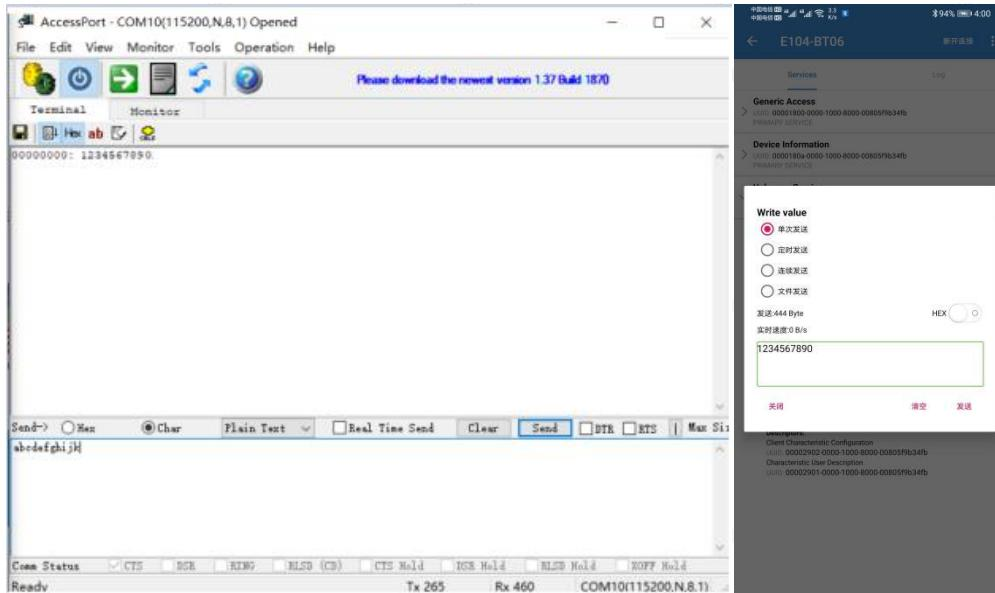
5. The effective data sent by the module to the mobile phone is "1234567890" (ASCII). At this time, the mobile phone receives the data as "123456789" such as:
