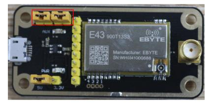
As shown in the figure, when the jumper cap is plugged in (select 5V power supply, mode 0), both E43-900TB-01 are configured in this way. When the corresponding serial port is opened, the data can be sent and received, and the AUX lamp flashing on the floor can be observed.
