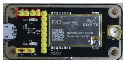
As shown in the figure, plug in the jumper cap (select 5V power supply, mode 3). Refer to the corresponding serial module manual for specific functions.
