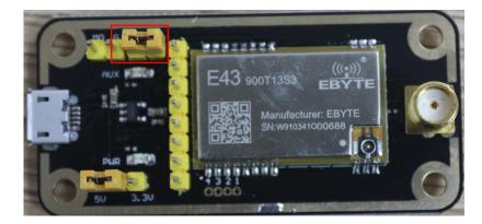
As shown in the figure, plug in the jumper cap (choose 5V power supply, mode 1). Refer to the corresponding serial module manual for specific functions.
