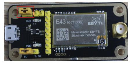
As shown in the figure, plug in the jumper cap (choose 5V power supply, mode 2). Refer to the corresponding serial module manual for specific functions.
